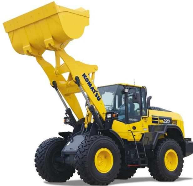
*Vilvoorde, December 2016* — Komatsu Europe presents the new WA320-8 wheel loader, an all-around utility performer for almost any worksite, with an attachment-friendly quick coupler, an EU Stage IV engine and up to 3 % lower fuel consumption.
